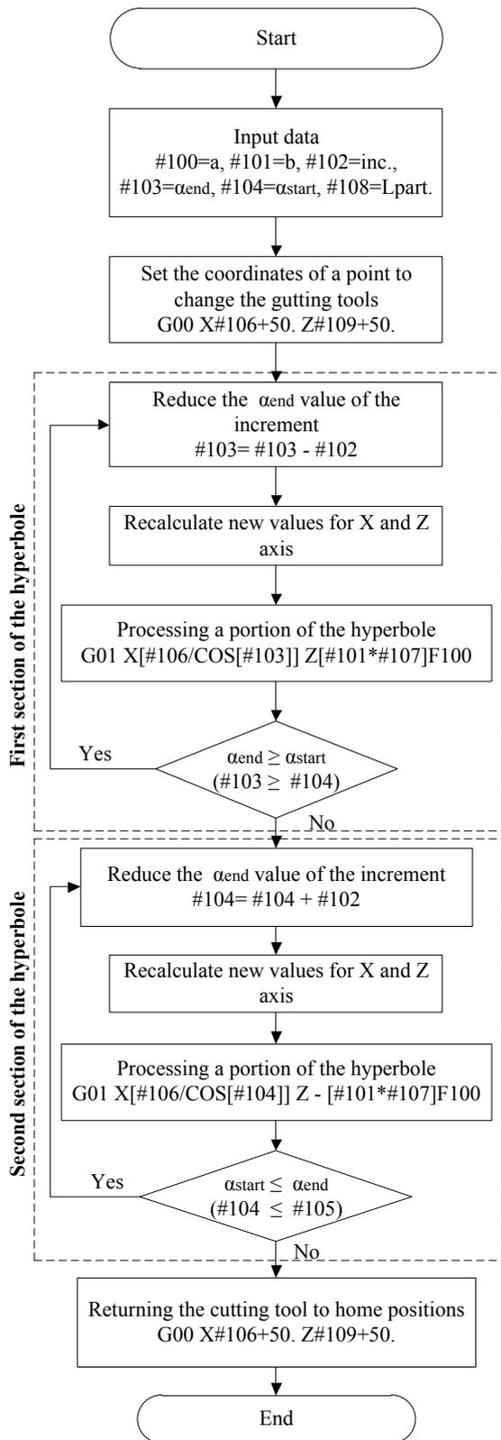
Fig. 5. Block diagram of the parametric (macro) program
