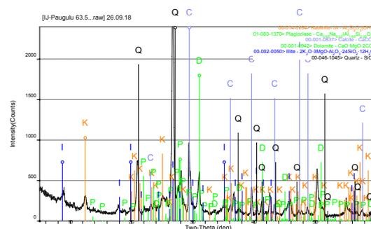
Fig. 3. X-ray diffraction pattern of clayey sample from lake Pauguļi, sampling depth 3.5 m. Minerals: Q – quartz, P – plagioclase, C – calcite, D – dolomite, I – illite, K – kaolinite.
