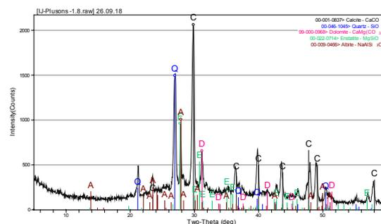
Fig. 4. X-ray diffraction pattern of clayey sample from lake Plusons, sampling depth 8 m. Minerals: Q – quartz, A – albite, E – enstatite, C – calcite, D – dolomite.
