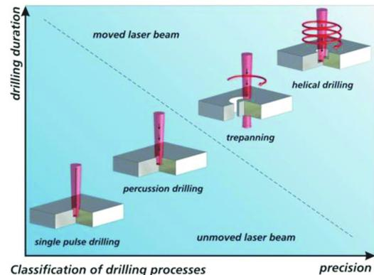
Fig. 3. Classification of drilling processes
