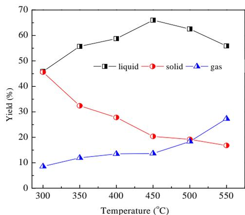
Fig. 2 Effect of temperature for cyanophyta pyrolysis
