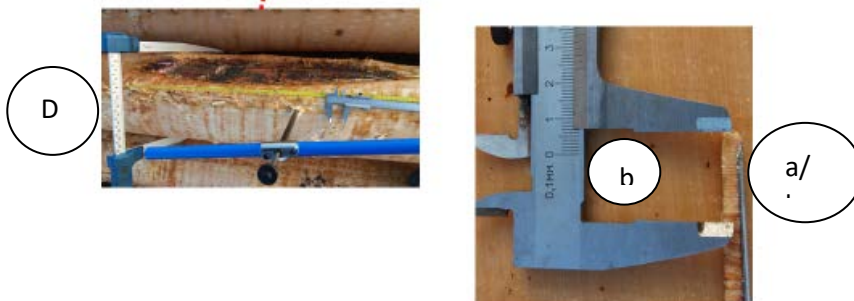
Fig. 6. The measurement example of side draught characterized parameters, where: A, B, C- zone of side draught position place; D_1 -wood pole diameter at side draught position, mm; b - side draught depth, mm; a/b - number/thickness of annual rings characterized the age of injury; L_1 - distance of side draught position measured from butt, cm; L - the length of wood pole, cm; D_1 - the wood pole top diameter, mm; D_b/D_{b0.5} - the wood pole (from B zone) butt diameter / the wood pole (from A zone) butt diameter measured 0.5m from the butt, mm
