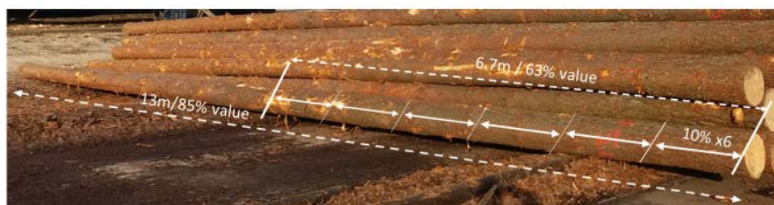
Fig. 5. The methodical distribution of pine stem by volume, zone and by timber value when stem length H- 24,5m, DBH -36cm; H/D=0.68
