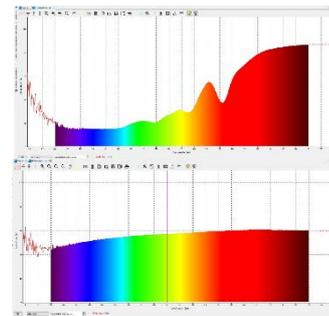
Figure 3b. The reflected light spectrum from the unmarked egg shell surface (above) and from the CO<sub>2</sub> laser marked egg shell surface (below).
