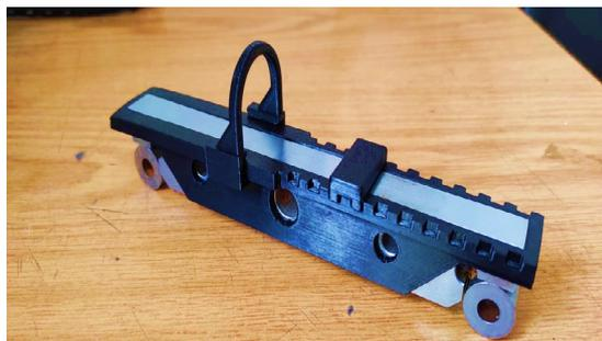
Fig.11 The device mounted on a 200mm sine bar.
