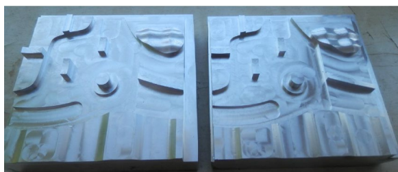
(a) detail 1 after finish milling by the variant without optimization (b) detail 2 after finish milling by the variant with optimization
