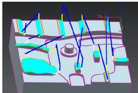
(c) spherical face cylindrical cutter with D = 10 mm.
