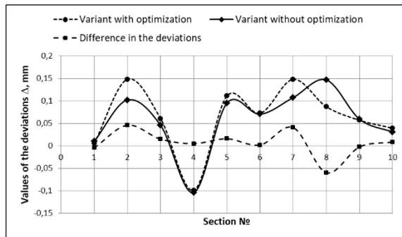
Fig. 9. Deviation in shape in points on the surface of a detail, processed both ways.
