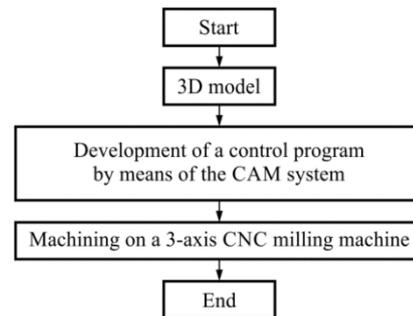
Fig. 1. Technological scheme for processing complex surfaces by milling, when using the Unigraphics system.
