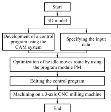
Fig. 2. Technological scheme for processing complex surfaces by milling, while using the developed PM.
