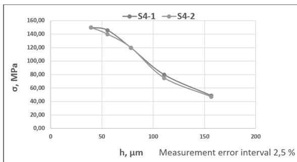
Fig. 3. Optimal distribution of the residual stresses along the depth of the surface layer of the workpieces, where S4-1 and S4-2 illustrates the optimal distribution of the residual stresses along the depth of the surface layer of two workpieces, processed under the given modes;  $h$  - depth of the studied material.
