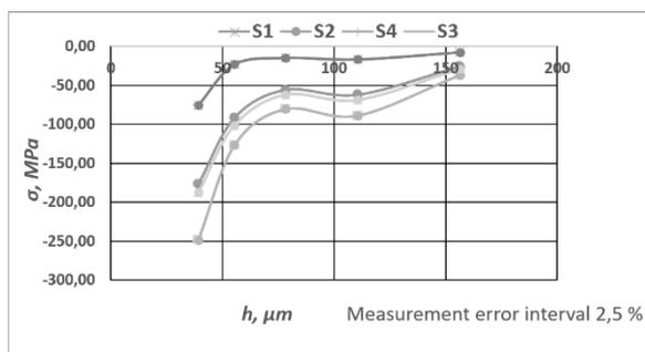
Fig. 2 Distribution diagram of the residual stresses, where S1 illustrates the stresses, measured in the original sample after heat treatment; S2 – in a heat-treated sample after the first spinning; S3 – in a heat-treated sample after the second spinning; S4 – in a heat-treated sample after the third spinning; h - depth of the studied material.
