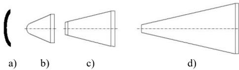
Fig. 1 Detail of AMg5, obtained after spinning in 3 transitions (the transitions are indicated by dashed lines) - a) original workpiece; b) first spinning; c) second spinning; d) third spinning.
