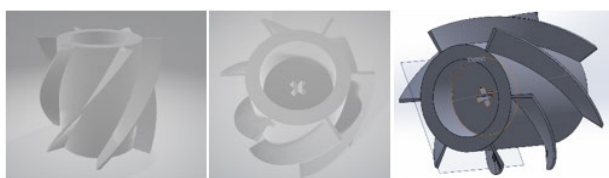
Fig. 4. Impeller with turned wings.
