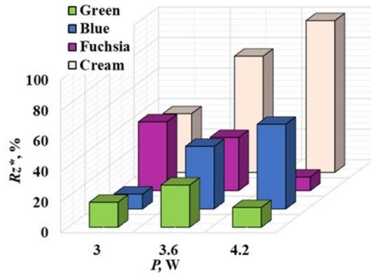
Fig.7. Surface roughness at average power changes.
