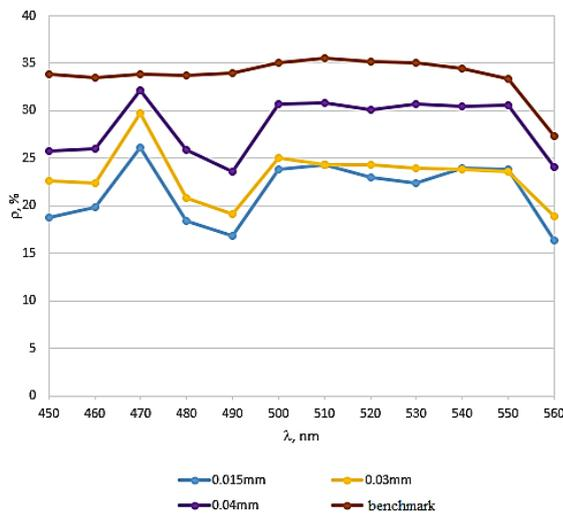
Fig. 7. Dependence of reflection coefficient as a function of wavelength for labelled samples at variable labelling step.
