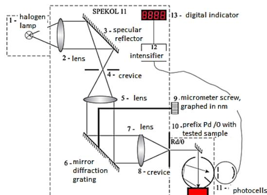
Fig. 5. Scheme of spectral reflection coefficient measurements with SPEKOL 11 spectrophotometer and attachment Rd/0.
