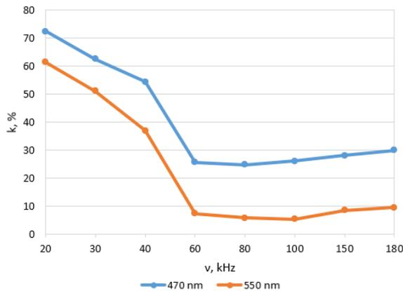
Fig. 10. Dependence of the contrast  $k$  of the mark on the frequency  $\nu$ , kHz for a sample of carbon steel C 75.
