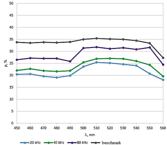
Fig. 8. Dependence of the reflection coefficient as a function of the wavelength for marked samples for the second experimental series.
