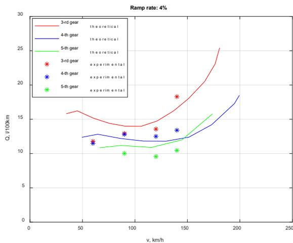
Fig. 9. Fuel consumption in third, fourth and fifth gear at 4% slope.
