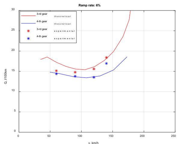
Fig. 10. Fuel consumption in third, fourth and fifth gear at 6% slope.
