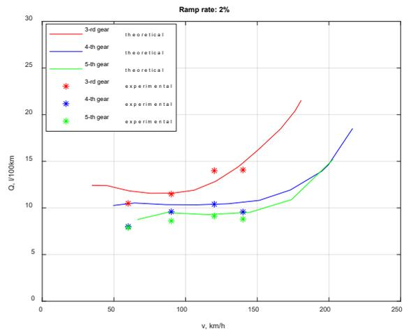
Fig. 8. Fuel consumption in third, fourth and fifth gear at 2% slope.
