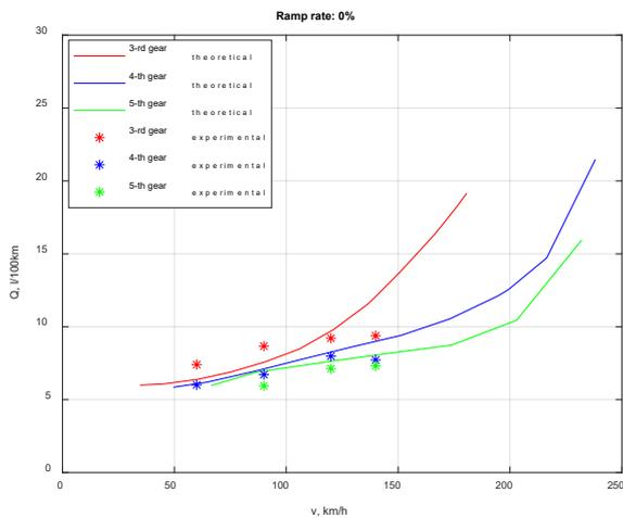
Fig. 7. Fuel consumption in third, fourth and fifth gear without a slope.
