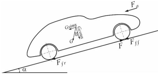
Fig. 1. Resistance forces acting on a moving car on a slope.
