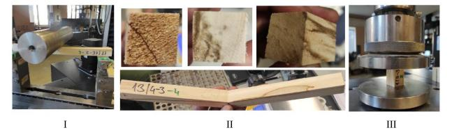
Fig. 6. The laboratory investigation process, where: (I)- 3. point bending strength and modulus of elasticity ISO 13061-3(4)-2014; (II)-testing samples; (III)- compression strength paralel to the grain ISO 13061-17-2017.
