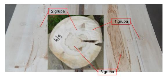
Fig. 5. Selecting of the testing samples according to the quality, where 1 grupa- sound timber, 2 grupa- heartwood coloured timber, 3 grupaheartwood hard rot stage timber.
