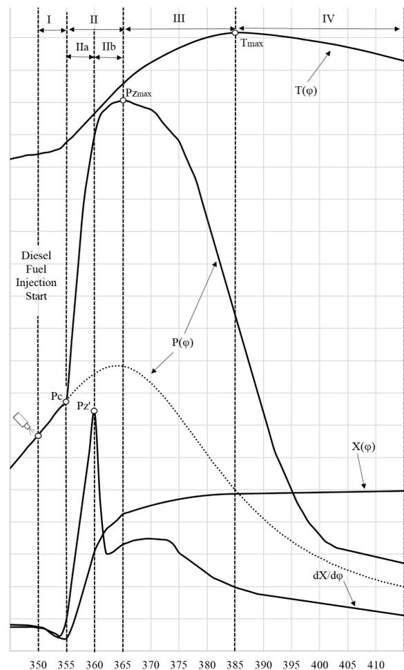
Fig. 1. Combustion parameters of compression ignition engines.
