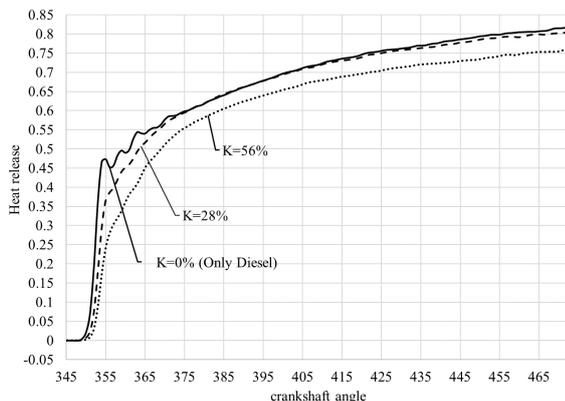
Fig. 4. Heat release of D3900 at 45% load and 1400 min<sup>-1</sup>.
