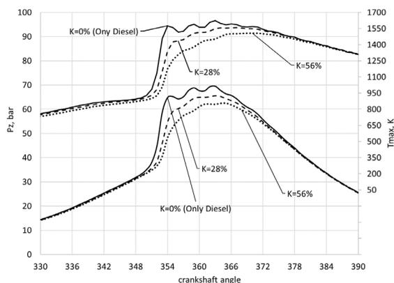
Fig. 3. Cylinder pressure and temperature of D3900 at 45% load and 1400 min<sup>-1</sup>.
