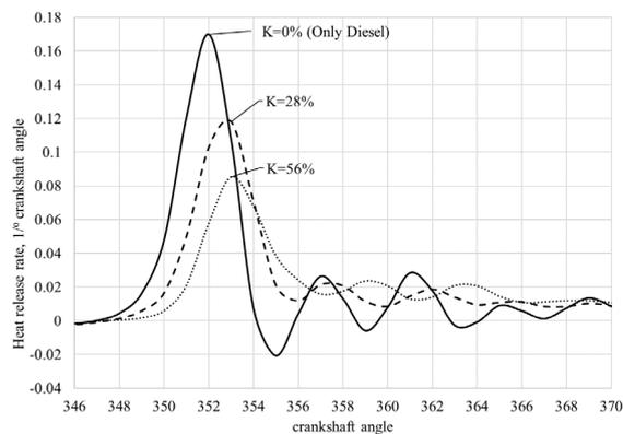
Fig. 5. Heat release rate of D3900 at 45% load and 1400 min<sup>-1</sup>.
