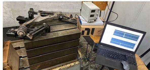
Fig. 6. Experimental determination of natural frequencies.
