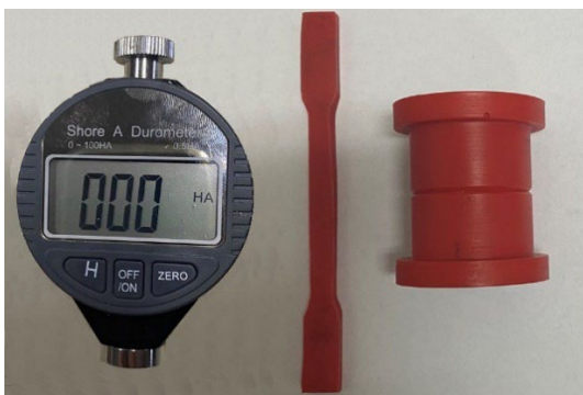
Fig. 2. Tester Shore A Durometer, specimen and bushing.
