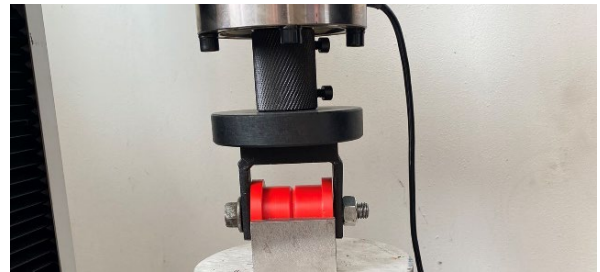
Fig. 7. Experimental compression test of polyurethane bushing.
