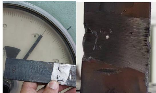
Fig. 9. Pores in samples No4 and No8.
