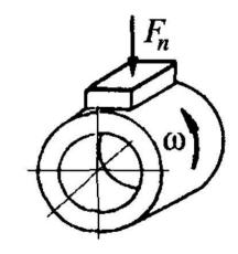
Fig.3 Timken test methods principal scheme
