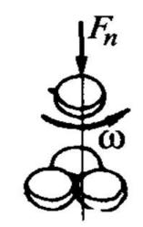
Fig.2. Four-ball test subassemblies principal block diagram
