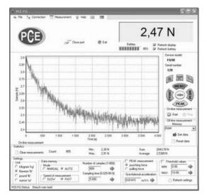
Fig.4. Dynamometer software screenshot
