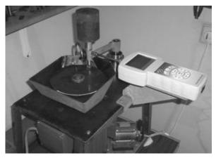
Fig.1 Oil additive testing machine
