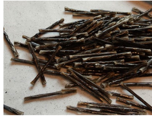
Fig.3. Prepared basalt Fibers 24 mm
