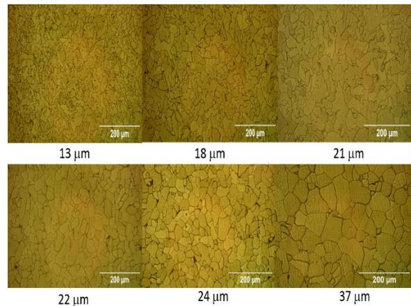
Fig. 2. Grain morphology after the heat treatment.
