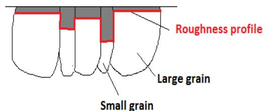
Fig. 7. Small v/s large grain ablation depth.
