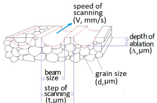
Fig. 3. Parameters of the laser ablation process.
