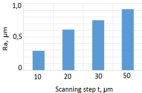
Fig. 5. The influence of the scanning step ( $t$ ,  $\mu\text{m}$ ) on the roughness of the samples (data for the scanning speed 150 mm/s).
