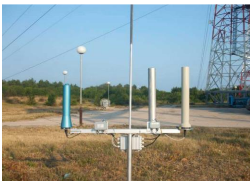
Figure 4: Photo of the upgraded sensors on an LMS. On the left is the spectrometry probe, in the middle is the start and on the right is the new dosimetry probe
