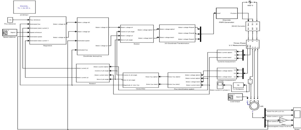
Fig. 2. Simulation model of FOC system with PWM
