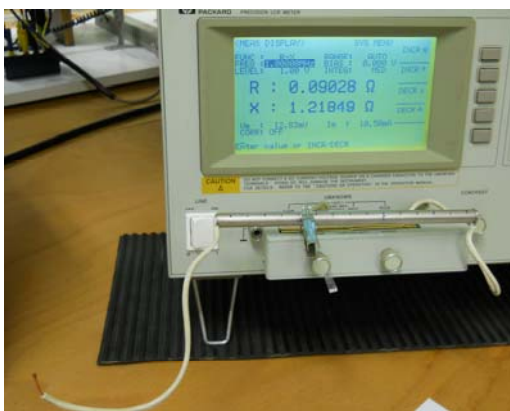
Fig.6. HP 4284A 20Hz- 1MHz LCR meter with the connected steel tube, resistance of the 10 cm long section is measured
