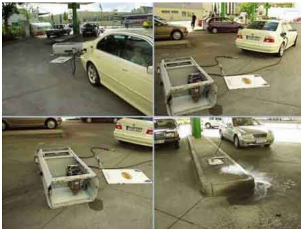
Fig.1. The accident that occurred due to not pulled out of a tank a filling pistol
