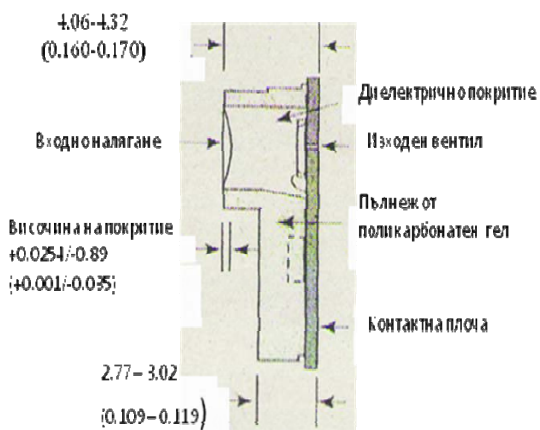
Fig.15. Principal scheme and photo of pressure sensor by Novasensor firm with application in the ecology
