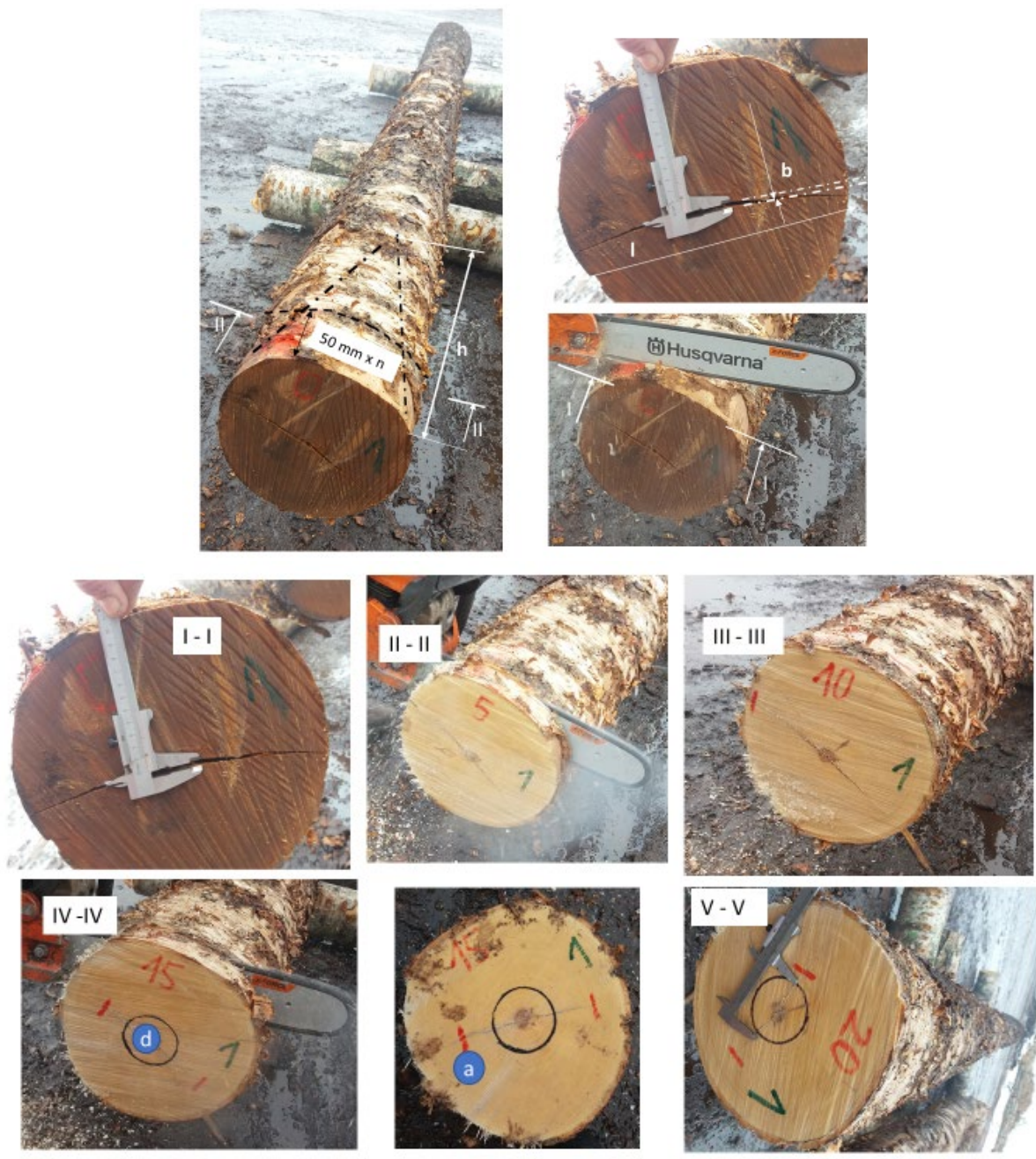
Fig. 4. Heart shakes distribution extending downward into the veneer log, where: (I-I); (II-II); (III-III); (IV-IV); (V-V) – end surface of veneer log; h- deep of the heart shake; b- width of the heart shake; l- actual length of the heart shake; d-diameter (70mm) of the residual cylinder; a- end point of the heart shake.
