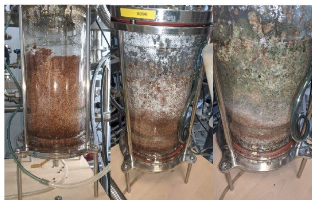
Fig. 6. T. harzianum Trichoderma SSF fermentation in wheat bran in static raimbault type column from left to right - 0h, 64h, 168h.
