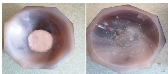
Fig. 4 Type of the sample reaction before and after milling during solid phase synthesis of [Mg(H 2 O)((H 2 N) 2 CO) 4 (SO 4 )].
