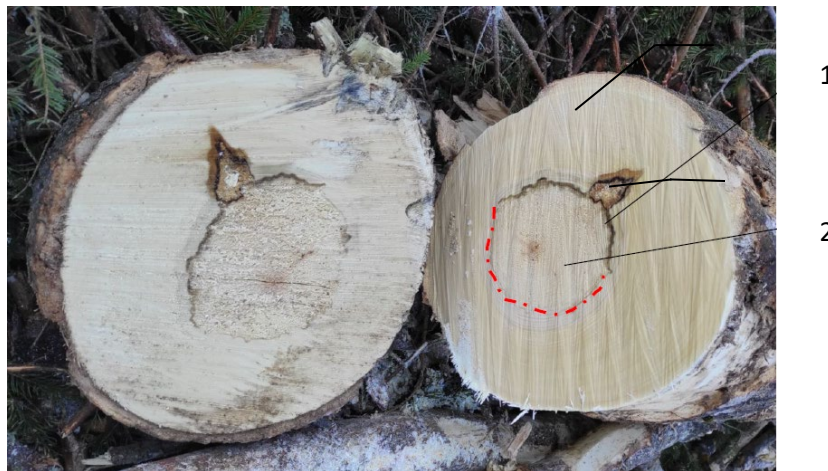
Fig. 7. The identification of the heartwood hard rot, where: 1- demarcation line; 2- the heartwood hard rot stage timber.
