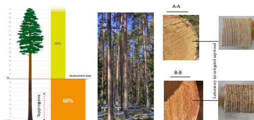
Fig. 6. The scheme of prepared samples from the trunk sapwood resinous zone and non-resinous zone.
