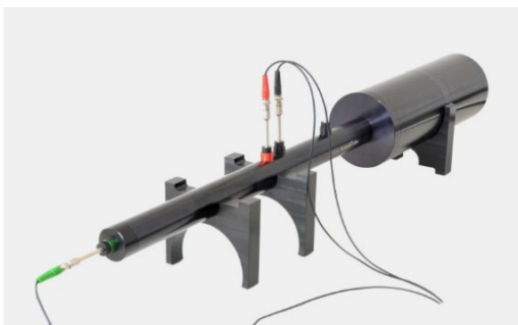
Fig.5. Sound Absorption impedance tube [10]
