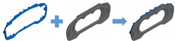
Fig. 2 Example of multi-component injection molding by layer-by-layer injection molding
