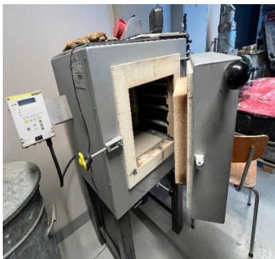
Fig.4. Oven setup for heat treatment
