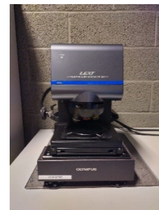
Fig. 1. Olympus LEXT OLS5000 3D Measuring Laser Microscope.
