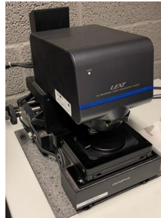
Figure 2: Photography of Lext 3D Laser Measuring Microscope OLS 5000
