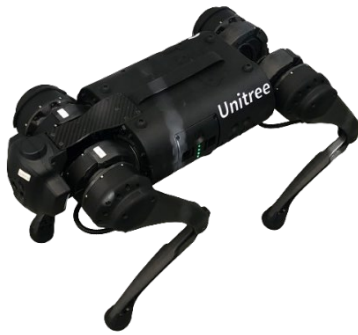
Fig. 1. Unitree Go 1 Edu quadruped robot.
