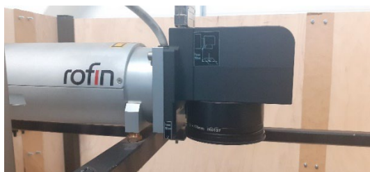
Fig. 1. Fiber laser Rofin PowerLine F-20 Varia.
