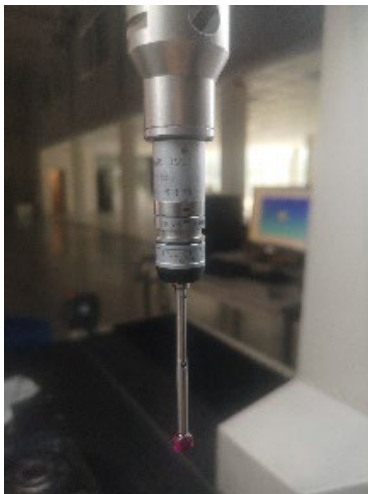
Fig. 2. TP20 sensor with D6 probe.
