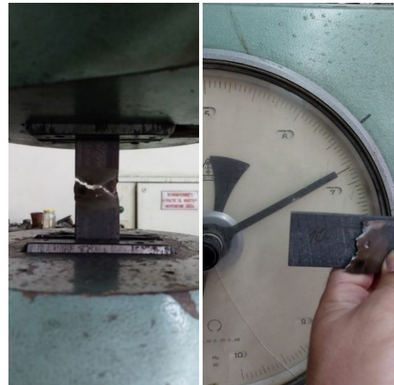
Fig. 5. Destruction of samples and checking the values.
