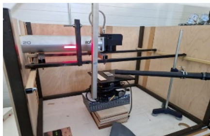
Fig. 1. Rofin powerline f 20 marking fibre laser system
