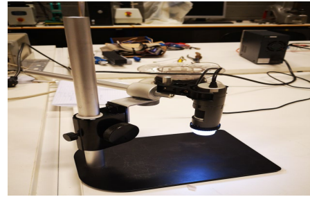
Fig. 2. Dino-Lite Edge AM7115MZT digital microscope.
