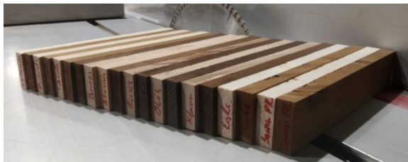
Fig. 1. Ten wood samples both before and after thermal treatment.
