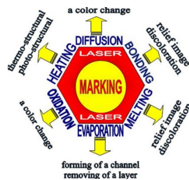
Fig. 1. Different physical processes by interaction of laser beam with the substrate [1]
