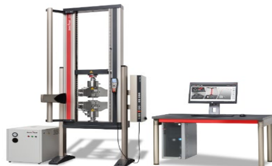
Fig. 4. Zwick / Roell Z150 material testing machine [25]
