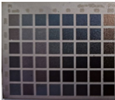
Fig. 5. Raster marked sample of stainless steel at different speeds and powers
