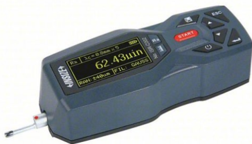
Fig 4 . Portable roughness tester INSIZE ISR – C002 [9].
