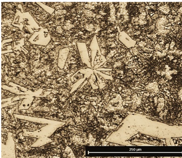
Fig. 2. Microstructure of AlSi21Cu5Cr alloy (pure metals)
