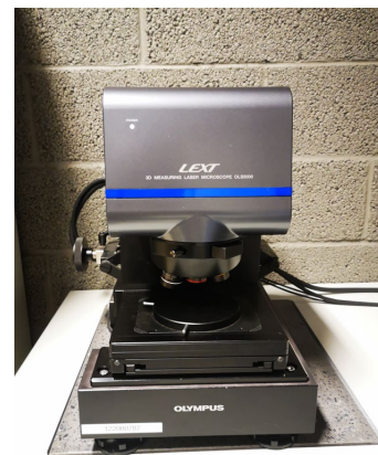
Fig. 3. Olympus LEXT OLS5000 3D Measuring Laser Microscope.
