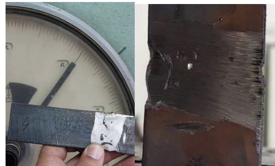
Fig. 9. Pores in samples No4 and No8.
