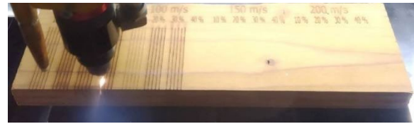
Fig. 5. Photograph of a thermally treated radiata wood sample engraved according to the created matrix.
