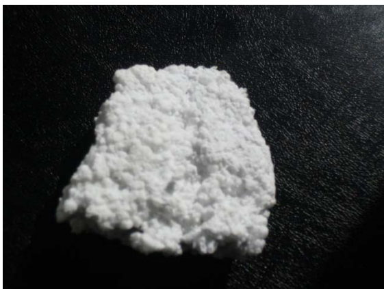
Fig. 1. Foamed polystyrene particles are bonded with cellulose fibers.
