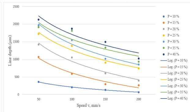
**Fig.6. Graph of line depth values on pine wood depending as power change.**
