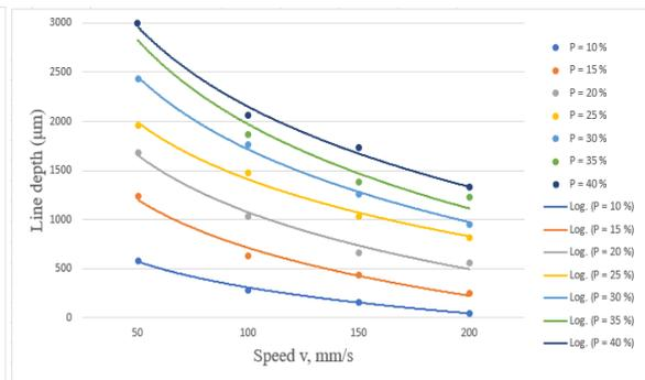
**Fig.4. Graph of line depth values on plywood material depending as power change.**
