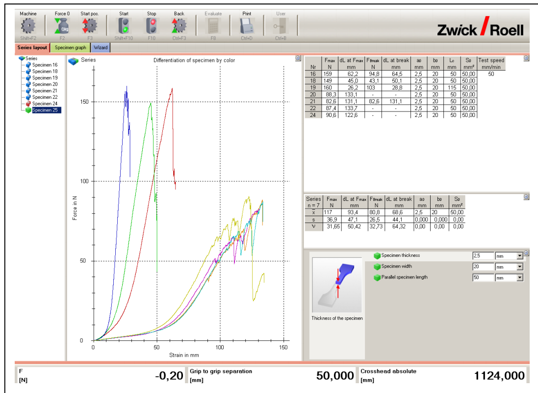
Fig. 5. The tensile test results of non – engraved examples (test speed v = 50 mm/ min).
