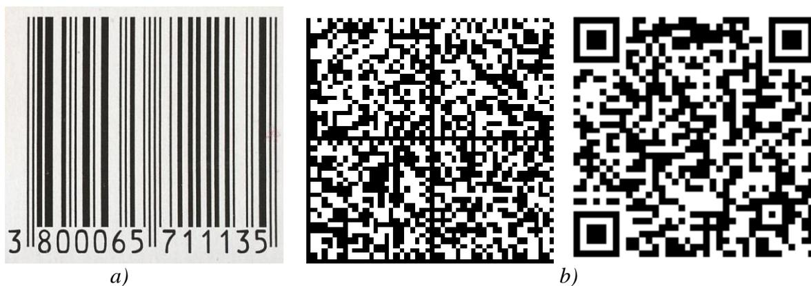
Figure 2 Marking of barcodes: a) 1D; b) 2D.
