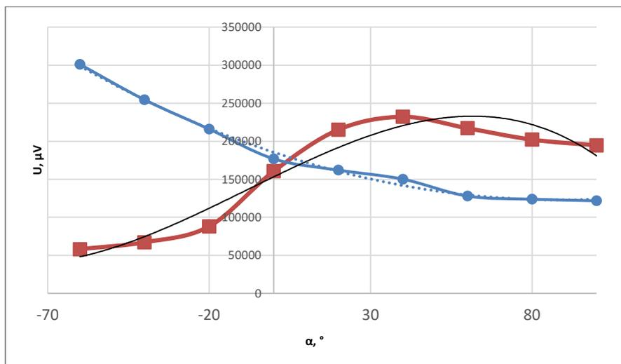
Figure 3 Strain sensors calibration curves. Red – dorsal sensor; blue – palm sensor
