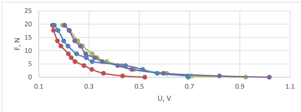
Figure 2 Pressure sensor calibration curves. Red – index finger, blue – thumb, purple – ring finger, green – middle finger
