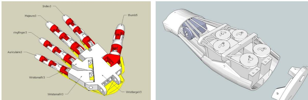
Figure 1 Robot – humanoid hand design (Langevin, 2017)
