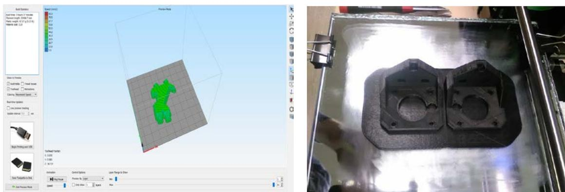
Figure 2 Robot – humanoid parts production by 3D FDM printing (created by authors)
