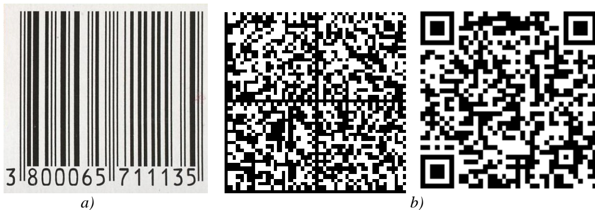
Figure 2 Marking of barcodes: a) 1D; b) 2D. (Sources: Pontius, 2012; Adams, 2014)
